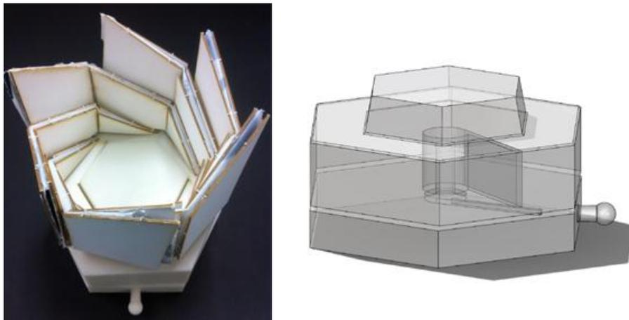
**Figure 4. (left) Prototype of the torsion spring test base with array. (right) Translucent rendering of CAD model, showing the cavity for the torsion spring**
