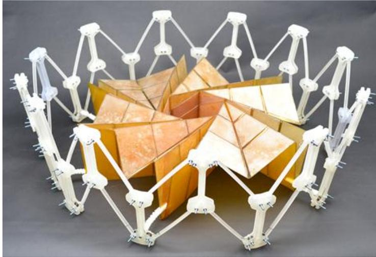
**Figure 2. Partially opened model of the array and truss**
