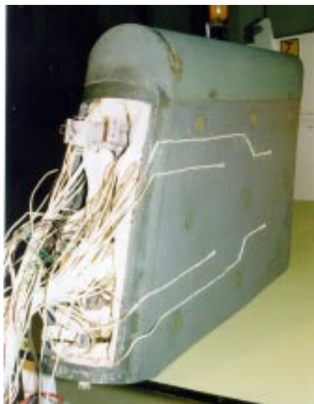
Fig. 6 Rudder, prepared for thermal-, mechanical - and kinematical test at DLR -Germany
