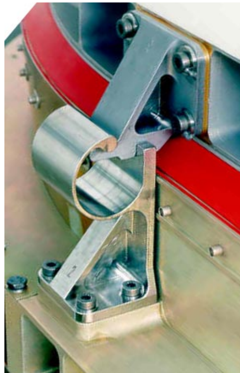
Figure 7. Flexible hinge mechanism, lateral view.
