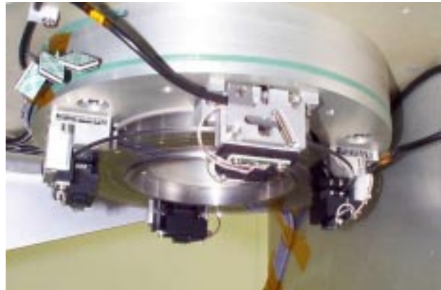
Figure 4: Flexural hinge-encoder assembly
