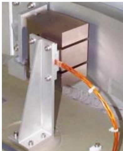
Figure 6: E-shaped voice coil actuator
