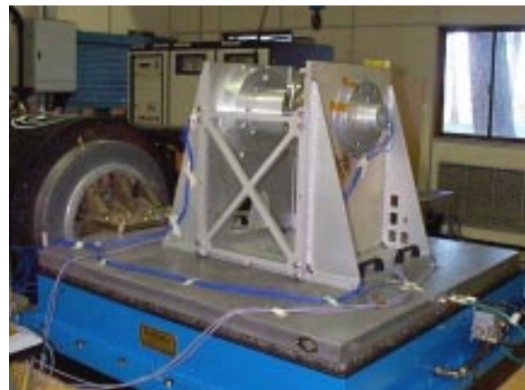
Figure 15: BBM instrumented for vibrations
