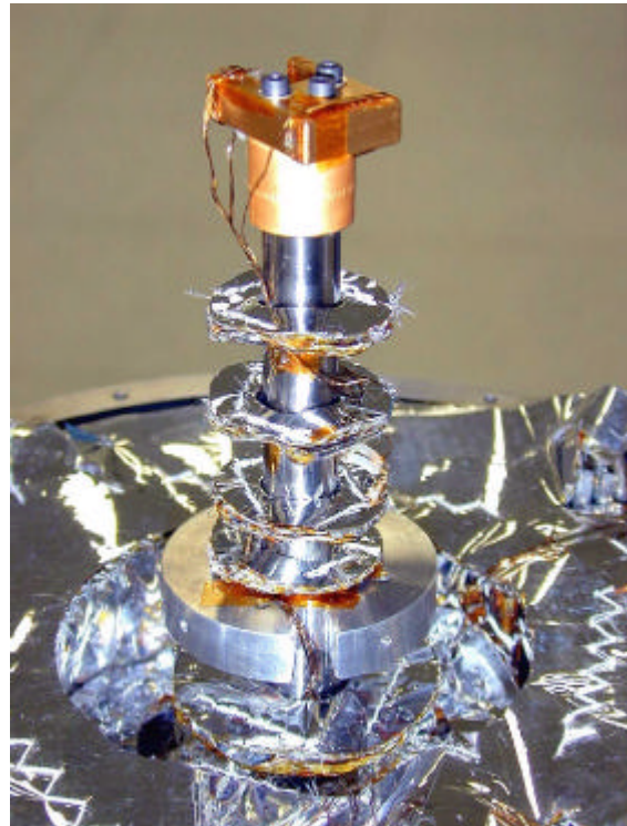
Figure 3. 10 K Cooler Cold-Tip with Temperature Monitor
