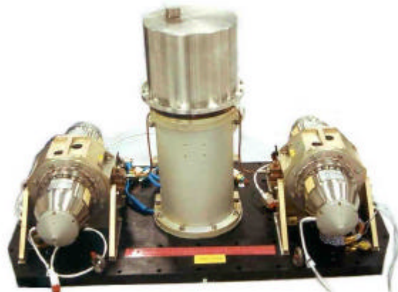
Figure 1. 10 K Closed Cycle Stirling Cooler System
