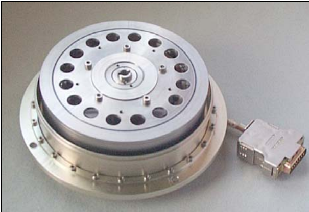
Figure 4: Prototype of the New Wheel Generation 0.2 – 1.6 Nms (top cover removed)
