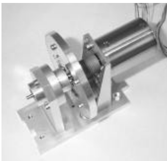
Figure 2 Wheel Assembly (note a metallic cover protects the wheel facets during build and test)
