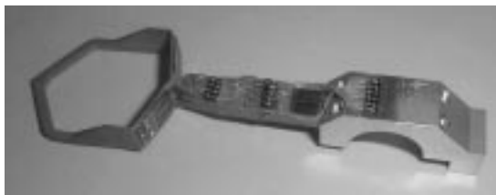
Figure 7: POD arm with bonded gauges
