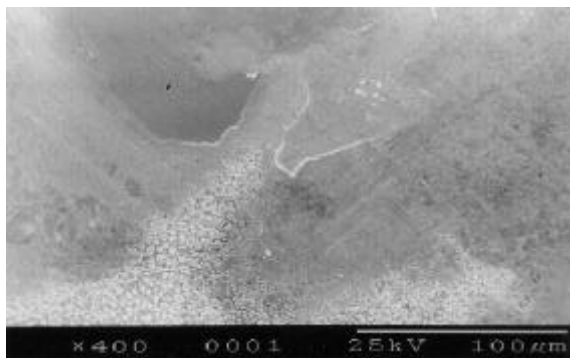
Figure 8 Scanning Electron Micrograph of the Edge of elliptical Zone of Lead lubricated Raceway shown in Figure 7
