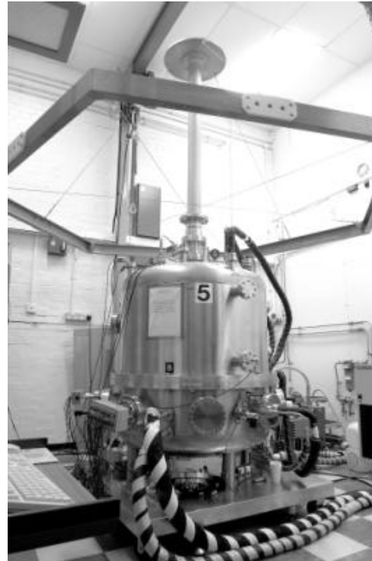
Figure 5: Solar Array Simulator above Thermal Vacuum test chamber
