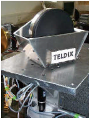
Figure 3: CMG momentum wheel under lifetime tests at Teldix
