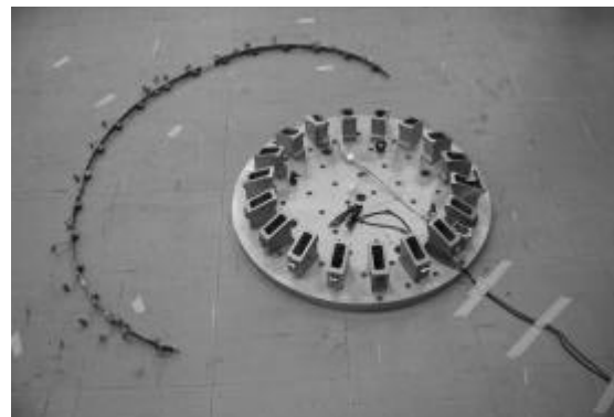
Figure 3-12 DM - Clamp Band release after vibration
