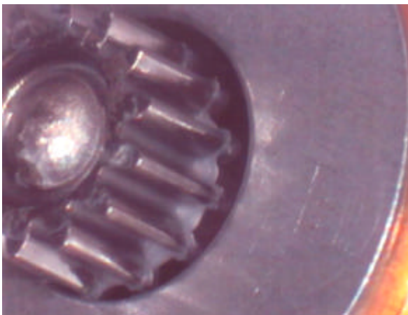
Figure 7: Maxon motor pinion following life-test
