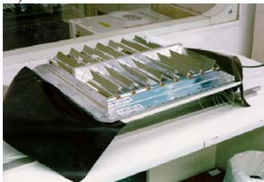
Figure 6, louvre assembly procedure . Final check of actuators calibration before functional test. Friction torque is checked in each blade.
