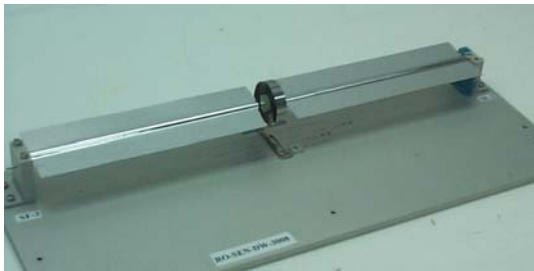
Figure 3, Blades and actuators are free to move during launch in the shaft direction. In the figure this subassembly is being calibrated before mounting.
