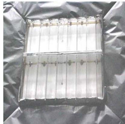
Figure 2, QM louvre instrumented for testing on the S/C.
