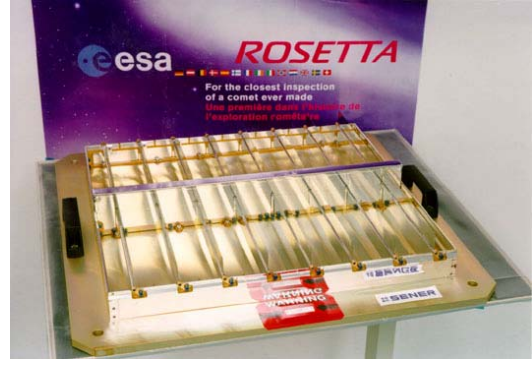
Figure 5, Eight actuators are inside the actuator housing in the centre of the louvre.
