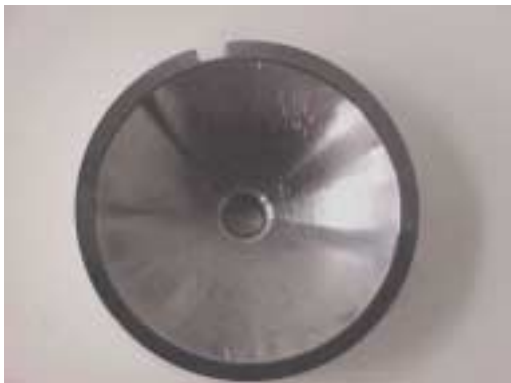
Figure 13 – Upper Fitting after 200 Cycles
