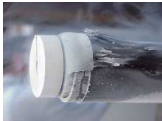
Figure 7 – Compression failure of unit at 77 K
