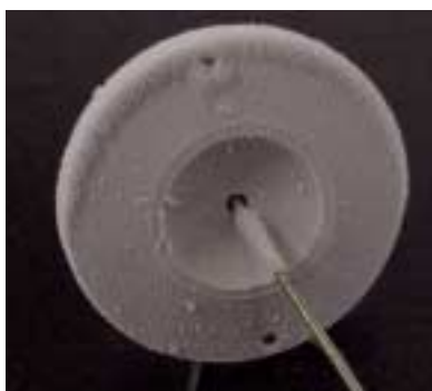
Figure 9 – Crystallised water on the helium tank interface fitting
