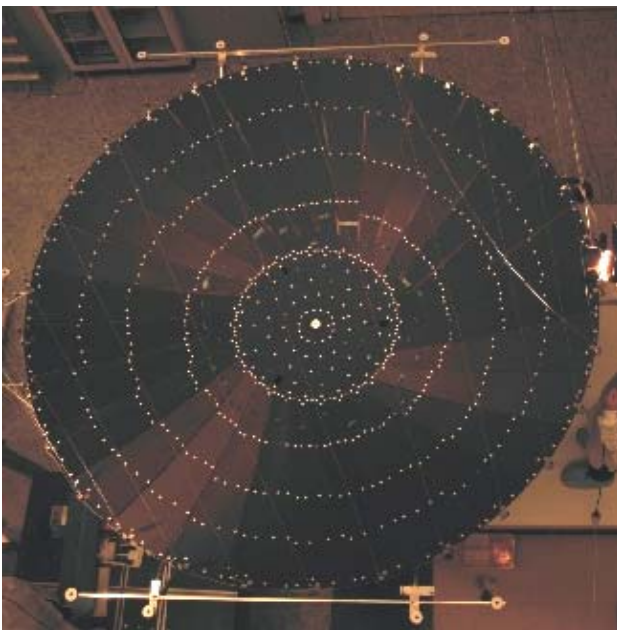
Fig. 13: Deployed Reflector during Contour Measurement.
