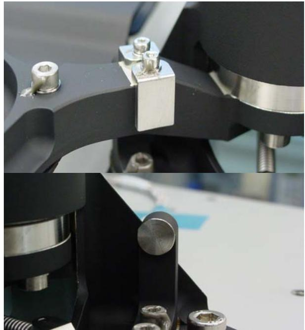
Figure 5. Mechanical end stops
