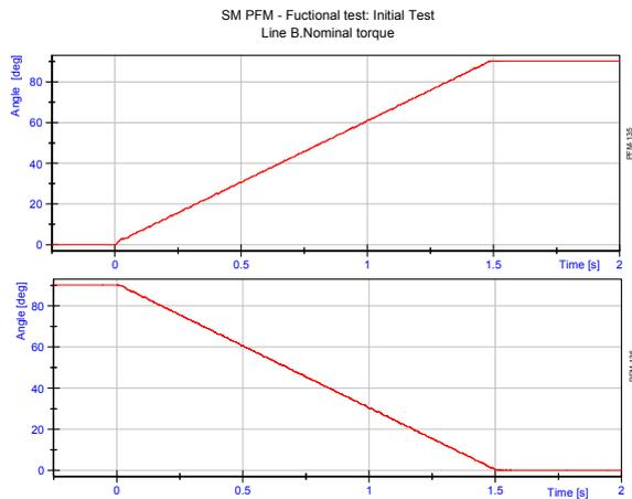
Figure 14. Position vs time open and close operations
