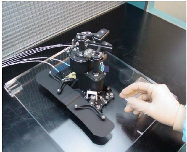
Figure 1. Pleiades Shutter Mechanism
