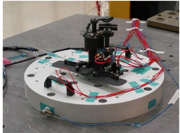
Figure 15. Test set-up for vibration test
