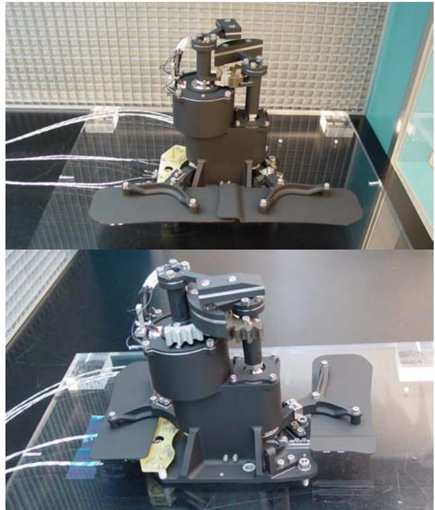
Figure 3. Shutter Mechanism in close and in open positions
