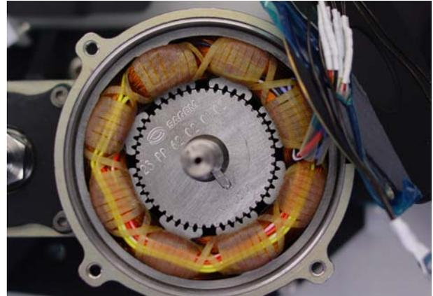
Figure 9. Motor rotor and stator
