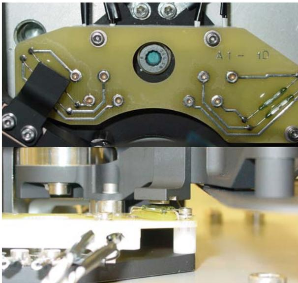
Figure 8. Reed switches PCB
