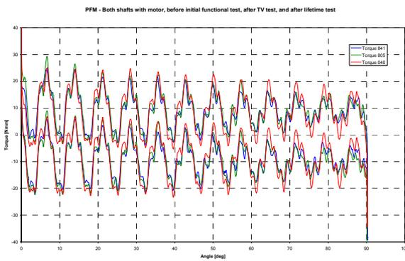
Figure 16. Resistive torque measurements
