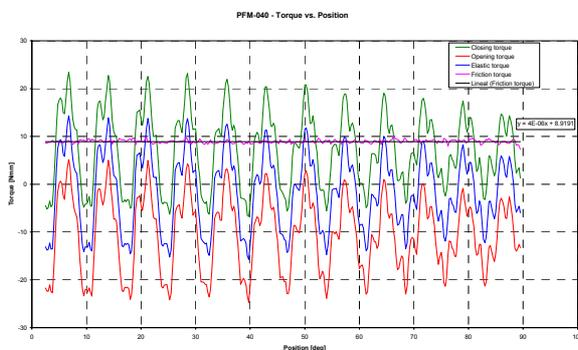
Figure 17. Resistive torque, friction and elastic contributions
