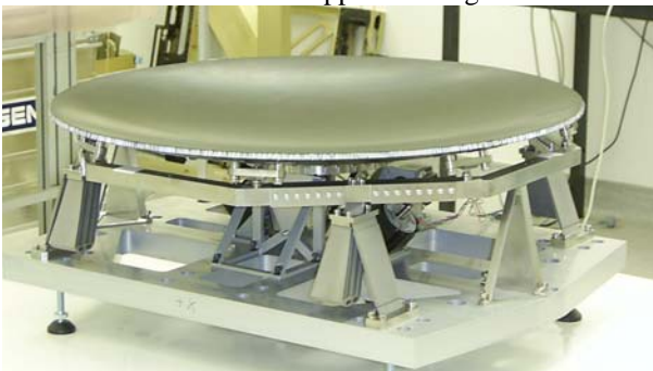
Figure 3. SubReflector Assembly configuration
