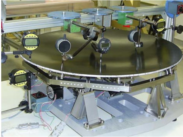
Figure 14. Dial gauges configuration for initial tests
