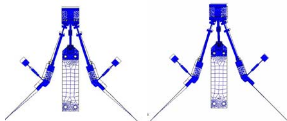
Figure 11. YZ Actuators for displacements in z direction and in YZ plane
