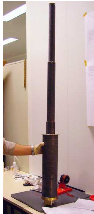
Figure 8: Engineering model first & second tube deployed
