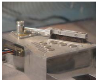
Fig. 3 (Top) Diagram of the rotary displacement of the wiper. (Bottom) Picture of the UV sensor with Dust wiper mechanism EM model.
