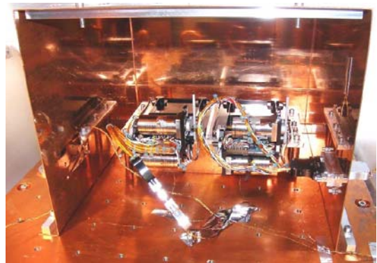
Figure 9: Picture of the CCC Qualification Model and Verification Model in the Cryogenic Thermal Vacuum Chamber at PSI.
