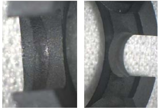
Figure 7. - Typical cage ball-pocket (left) and cage-land witness marks (right) following operation over 611 million revs
