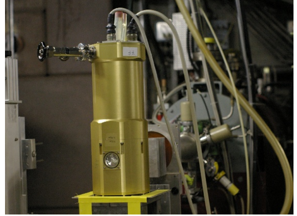
Figure 1. MPIA cryostat in the PIF laboratory. The magnet samples are inside the cryostat at cryogenic temperatures. The collimated proton beam enters the cryostat through plexiglass windows.
