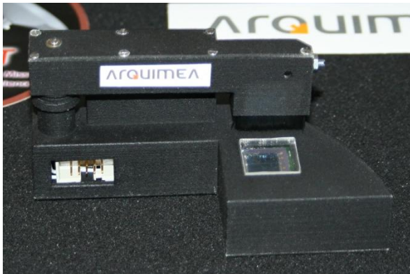
Figure 5: Front view of the SMA Rotary Actuator.
