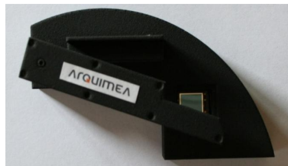
Figure 1. Top view of the SMA Rotary Actuator.
