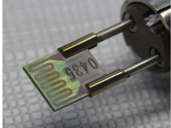
Figure 8 Thermal Knife after cutting tests
