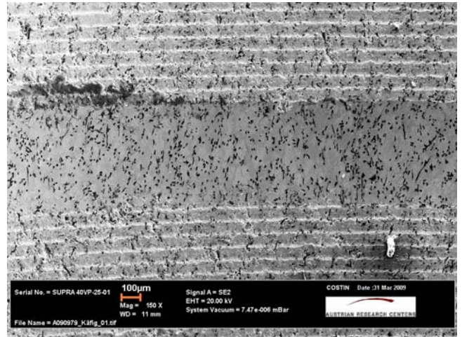
Figure 8: SEM-image: cage pocket with the grooves from manufacturing (bottom and top) and the track created by the balls.
