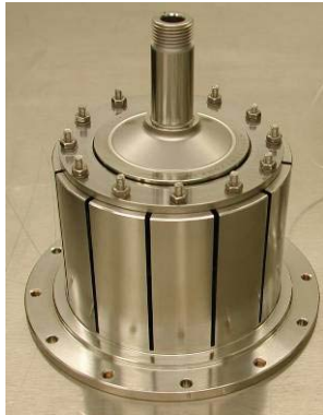
Figure 5. Isostatic Bearing Mount for Cryo Testing.
