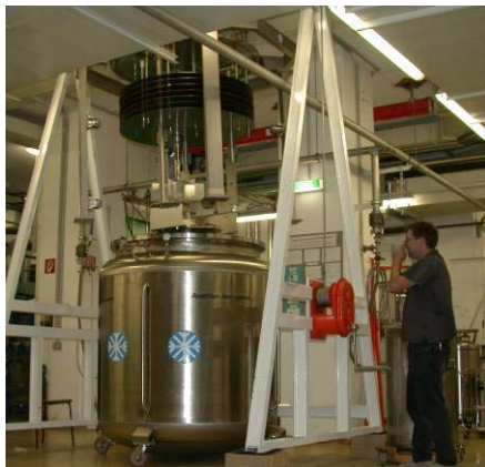
Figure 7. Insertion of the Cryostat Cover with the Unit under Test into the Cryostat.
