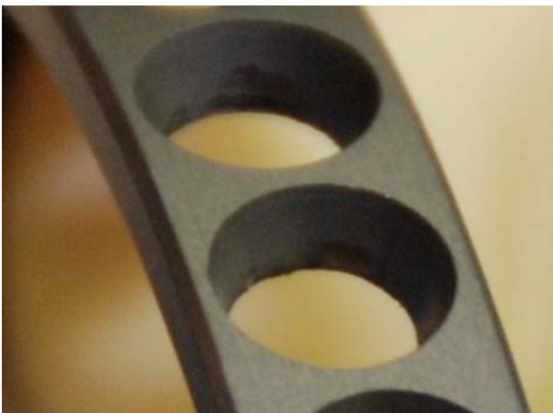
Figure 3. Wear Marks inside the Cage Pockets.
