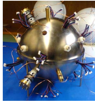
Figure 10: Stator and rotor integration
