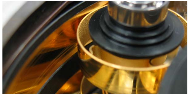
Figure 3: Contact surface finish after 3 million revolutions. The load bearing contact area has been deformed to a smooth, lustrous finish resulting in a more uniform contact interface.
