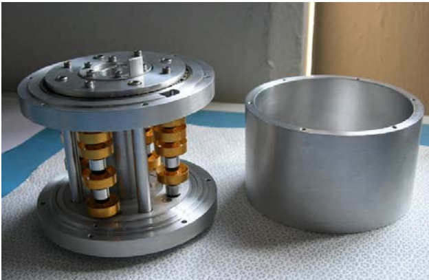
Figure 2. RCC Subassemblies (Dimensions: 4" height x 4.5" diameter)
