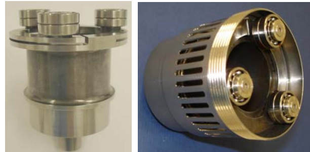
Figure 8.- Wave generator inside flexscrew with cut-outs in the threaded zone.
