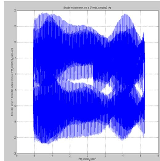
Figure 9. Encoder error versus reference metrology.
