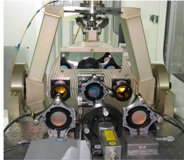
Figure 7. EBB functional assembly in the OGSE set-up.
