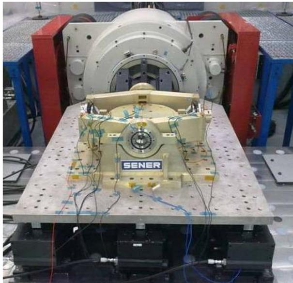
Figure 6. EBB MTG FCI SM in vibration test
