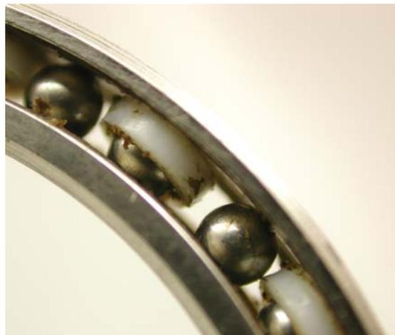
**Figure 7. Typical Bearing Lubricant, Post-Failure**
