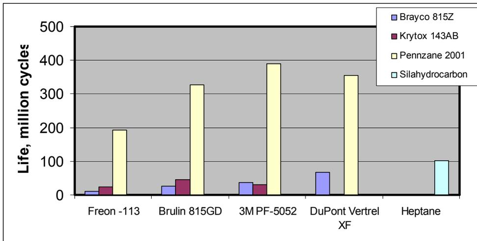
Figure 8. Effect of Cleaning Solvent on Average Bearing Life
