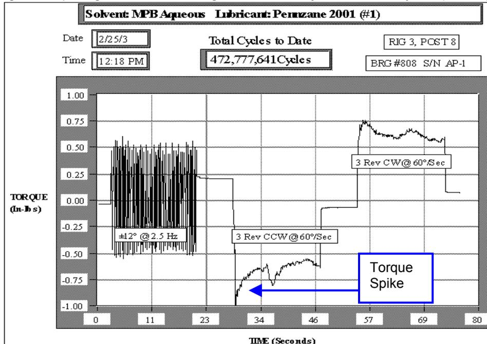
**Figure 6. Pennzane bearing torque trace approaching failure. Note torque spike of > 1 in-lb from debris bump at transition to 3 revs of continuous rotation**
