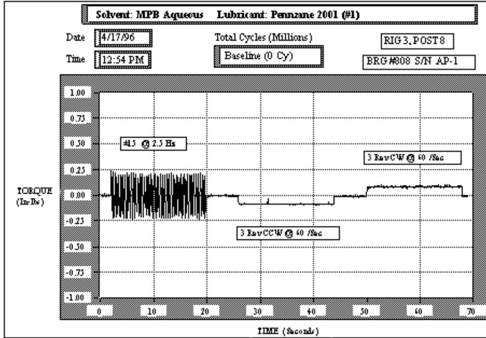
**Figure 4. Pennzane 2001 Bearing Torque Trace at 0 cycles**
