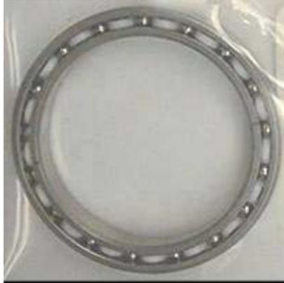
Figure 1. Test bearing with toroid ball separators
