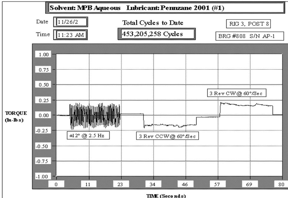
**Figure 5. Pennzane 2001 Bearing Torque Trace at 453M cycles**
