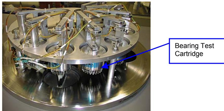
**Figure 2. Bearing life test fixture with individual strain gaged bearing cartridges**
