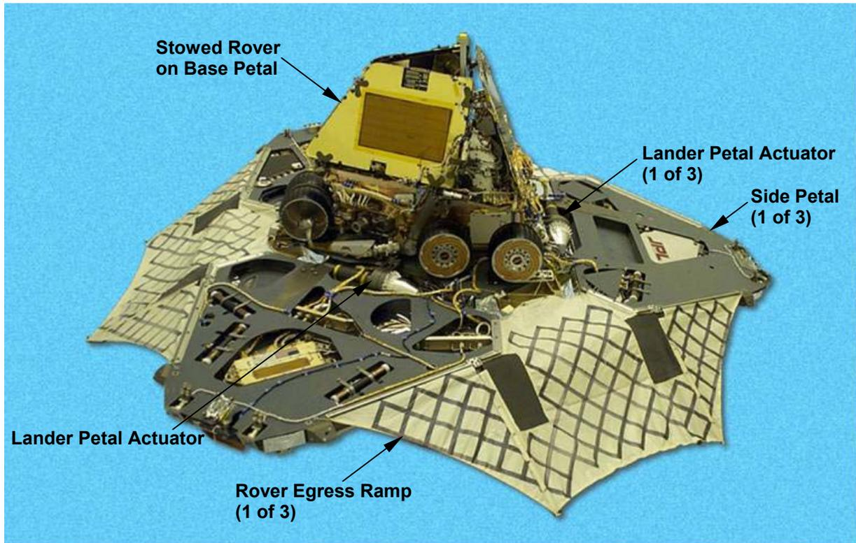
**Figure 1. Lander Petal Actuators open each MER Lander side petal to the iron cross position, where all petals are coplanar. Petal motion past this condition is called over-deployed.**
