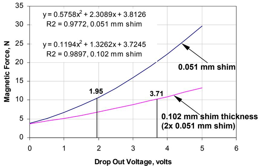
Figure 9. Regression curves from test data are appropriately shifted and used to determine the drop-out voltage required for a minimum 2.0 factor of safety.
