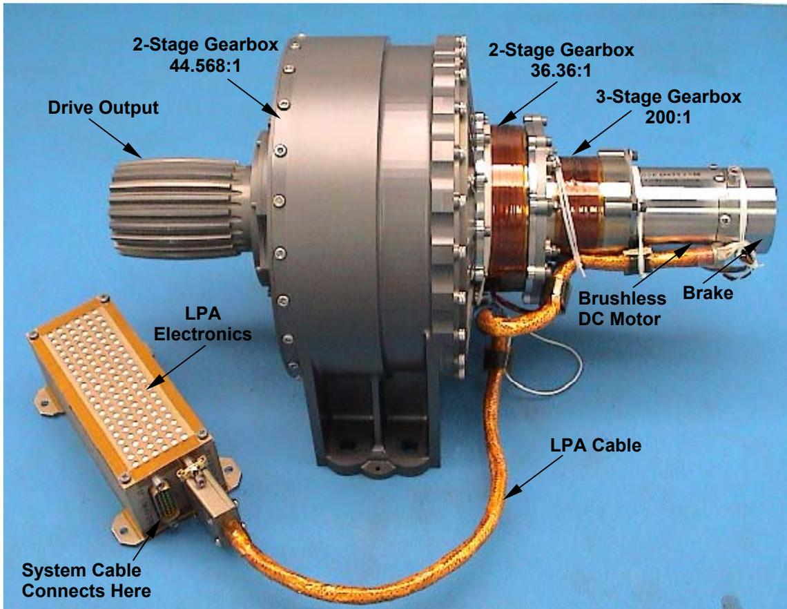
Figure 3. MER Lander Petal Actuator with its electronics
