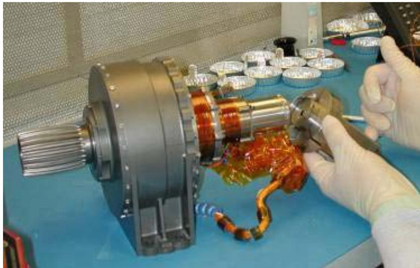
**Figure 10. The brake assembly is removed from the Lander Petal Actuator during rework to add an additional shim.**
