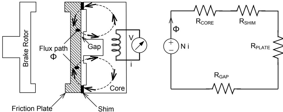
**Figure 12. Magnetic circuit model**
