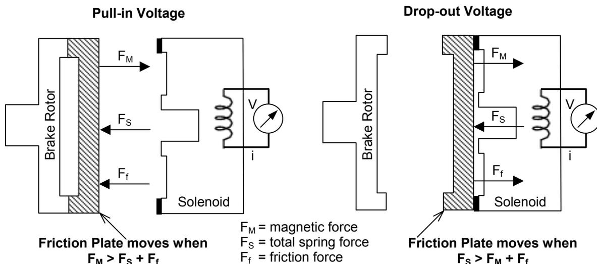
Figure 7. Force balance for brake pull-in and drop-out voltages
