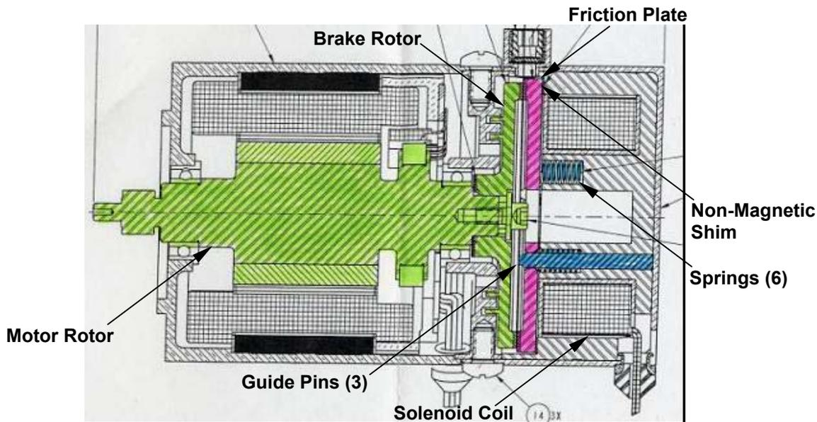
Figure 5. Cross-section of the Lander Petal Actuator motor/brake assembly
