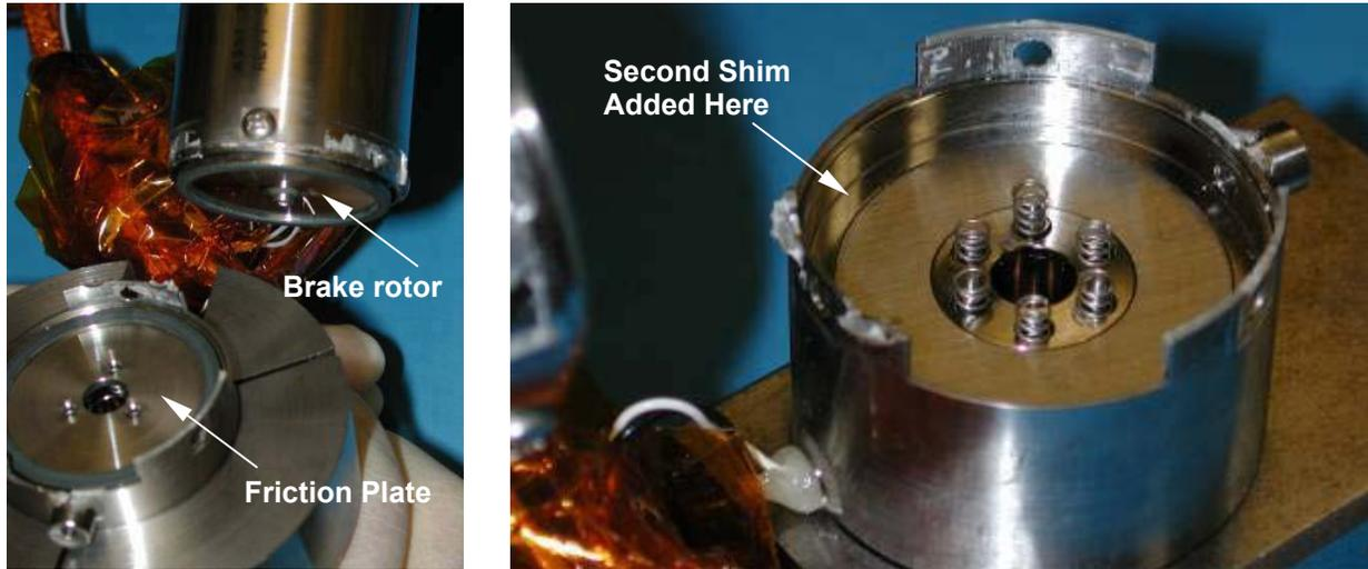
Figure 11a and 11b. Close-up views of the brake assembly during rework
