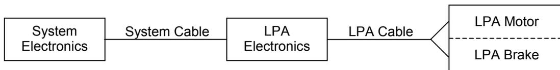
Figure 4. The LPA motor and brake are separately powered and commanded by the system electronics through the LPA electronics, a brushless motor drive electronics.
