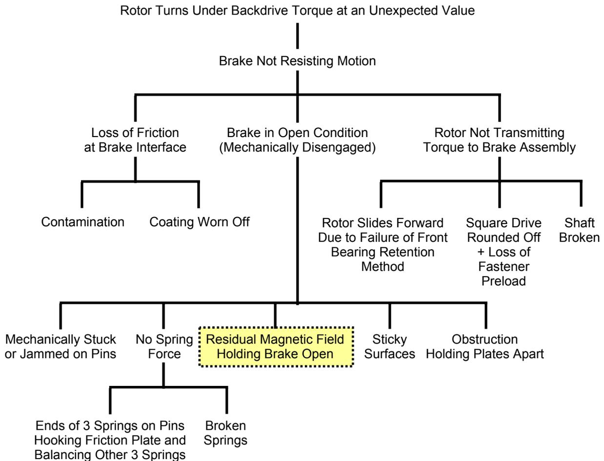
**Figure 6. Fault tree for LPA brake failure with the actual failure highlighted in the dotted box**
