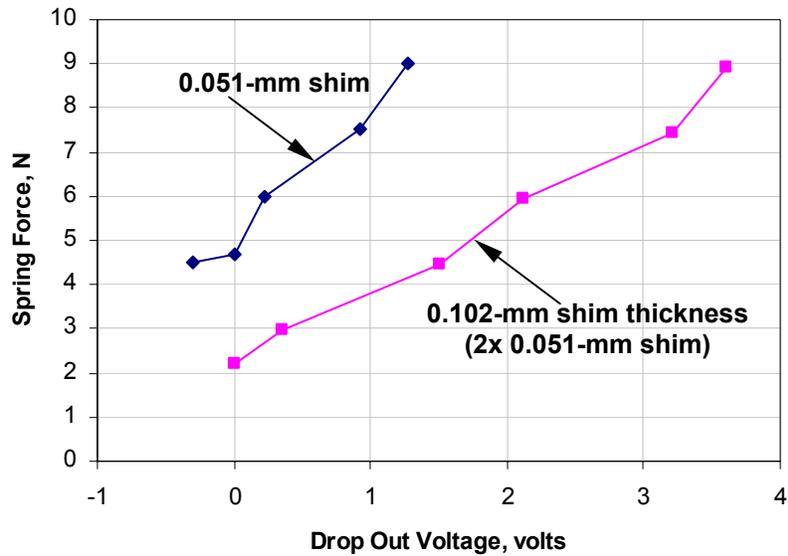
Figure 8. Test data from a spare brake assembly characterizes the variation of drop-out voltage with spring force for two different shim thicknesses.
