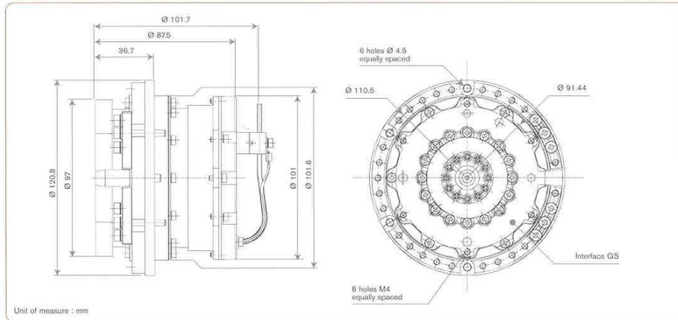
**Figure 3. SARA<sup>®</sup> 21 mechanical interface**
