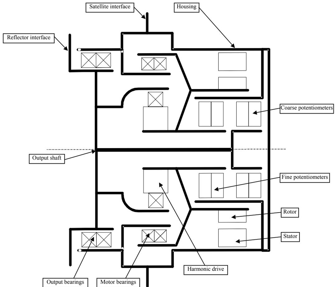
**Figure 4. SARA<sup>®</sup> 21 kinematic scheme**
