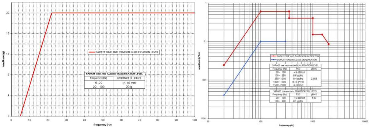
Figure 7. SARA<sup>®</sup> 21 sine and random vibrations levels
