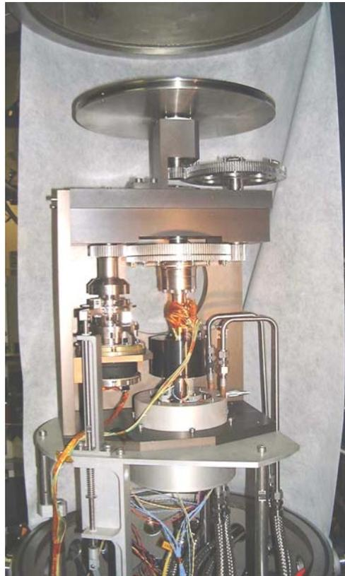
**Figure 10. SARA® 21 thermal vacuum life test set-up**
