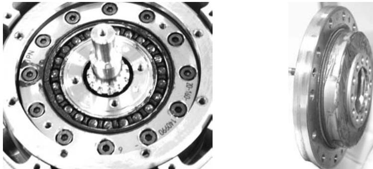
**Figure 11. SARA<sup>®</sup>21 QM CSD 20-160 Harmonic Drive after qualification tests**
