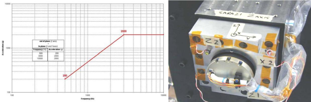
Figure 8. SARA<sup>®</sup> 21 shock level and test set-up
