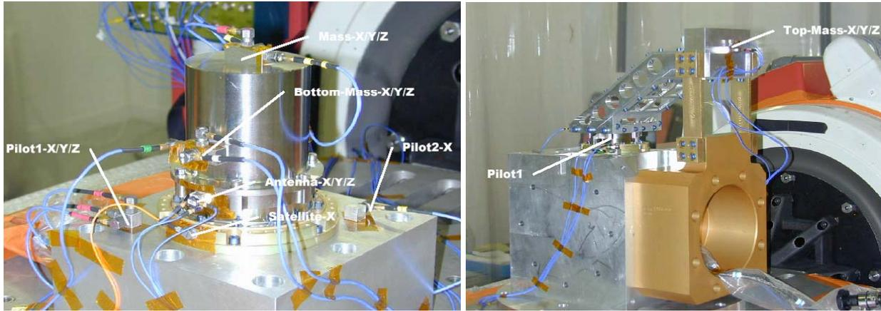
Figure 6. SARA<sup>®</sup> 21 vibration test set-ups (centered mass for sine and random + deported mass for torsion load)
