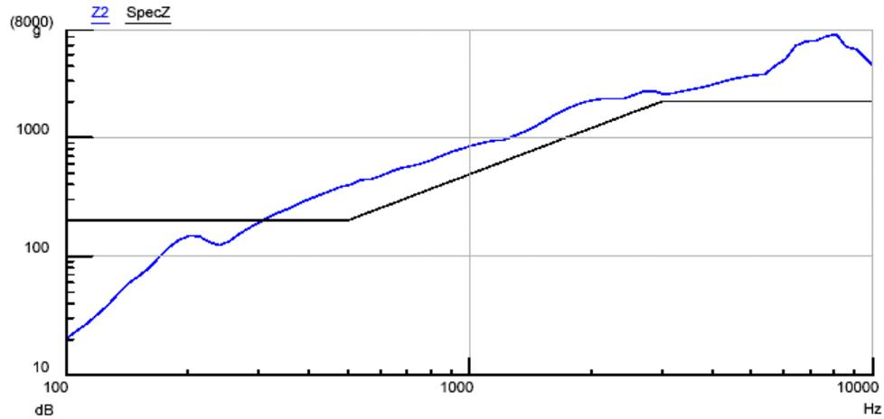
**Figure 9. SARA® 21 shock response spectrum along Z-axis**
