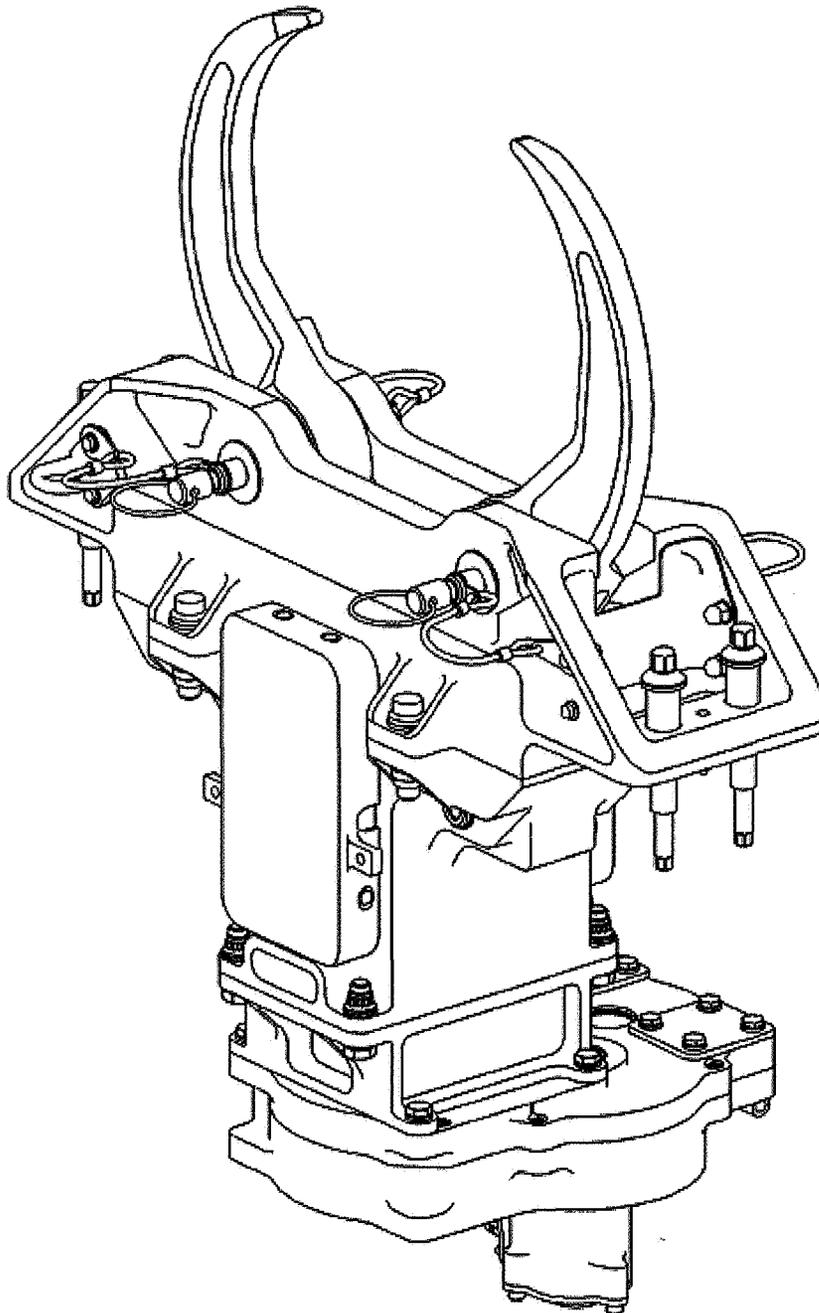
**Figure 3. ISS P1 Truss SSAS Capture Latch**
