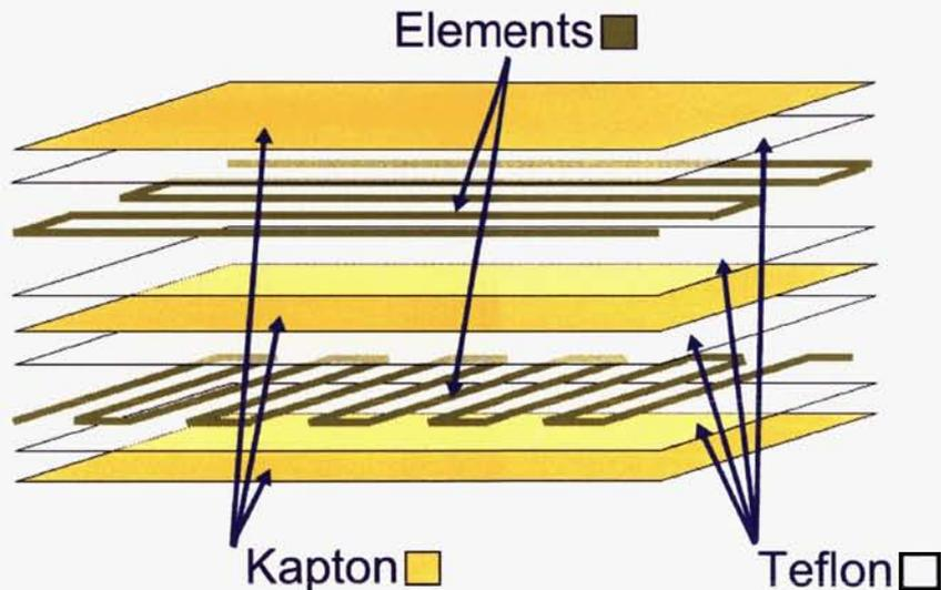
Figure 1. Layered Design Flexible Heater Exploded View
