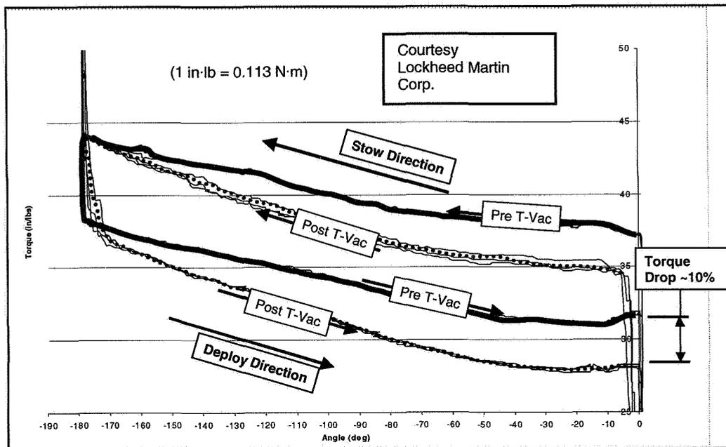
**Figure 3. Torque vs. Angle for 180-degree Hinge**
