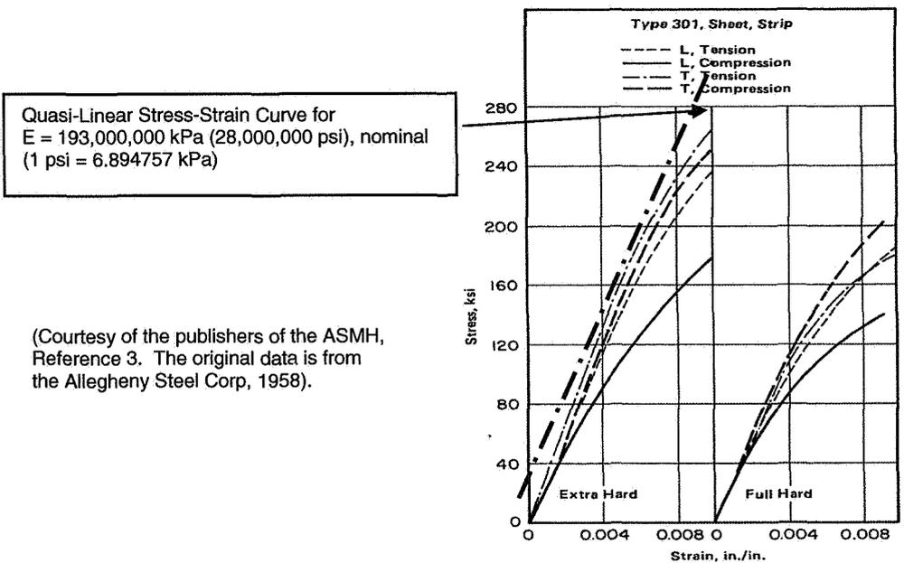
FIGURE 3.0212. STRESS-STRAIN CURVES FOR SHEET AND STRIP COLD ROLLED TO FULL-HARD AND EXTRA-HARD TEMPERS (11)
