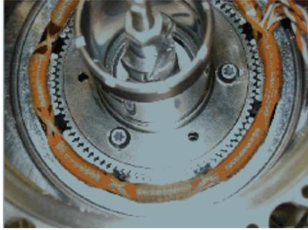
**Figure 8. Stepper motor and roller screw assembly**
