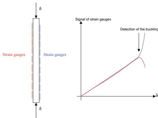
**Figure 15. Detection of the free flex buckling**
