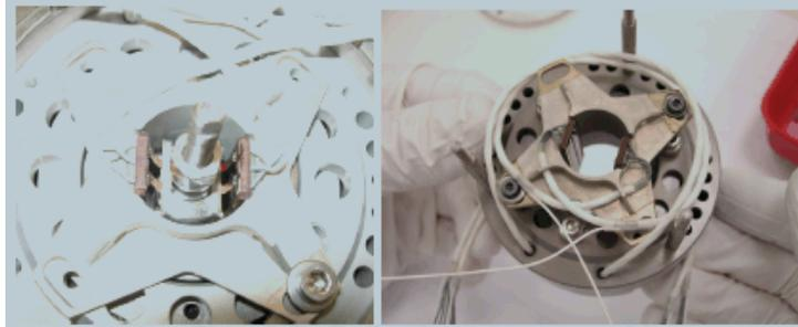
**Figure 5. Potentiometer assembly**
