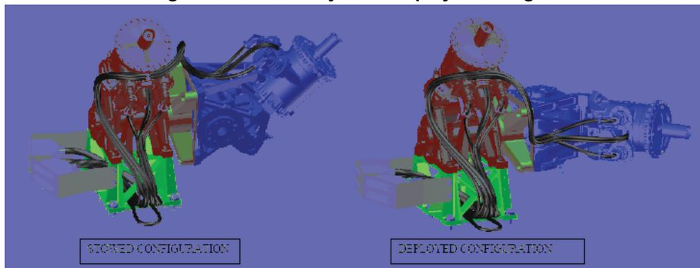
**Figure 3. MADPM stowed and deployed configurations**
