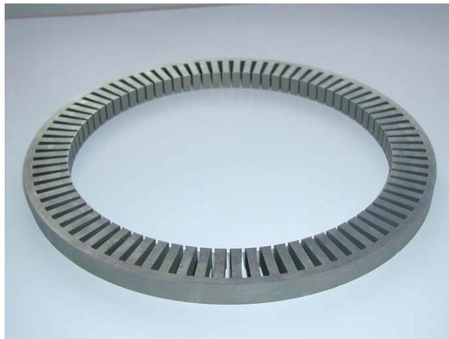
**Figure 8. Thin Sheet Stacking with Structural Bonding**
