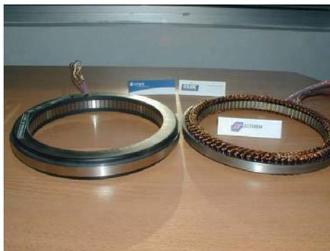
**Figure 7. Existing Referenced Stator and the Structurally Bonded Stack**
