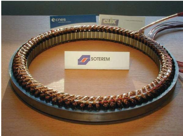
**Figure 1. Brushless DC motor stator : 18001-2 (SOTEREM)**
