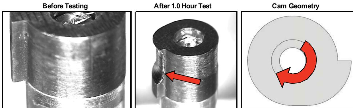
**Figure 5. 17-4 PH Prototype Cam Wear and Geometry**
