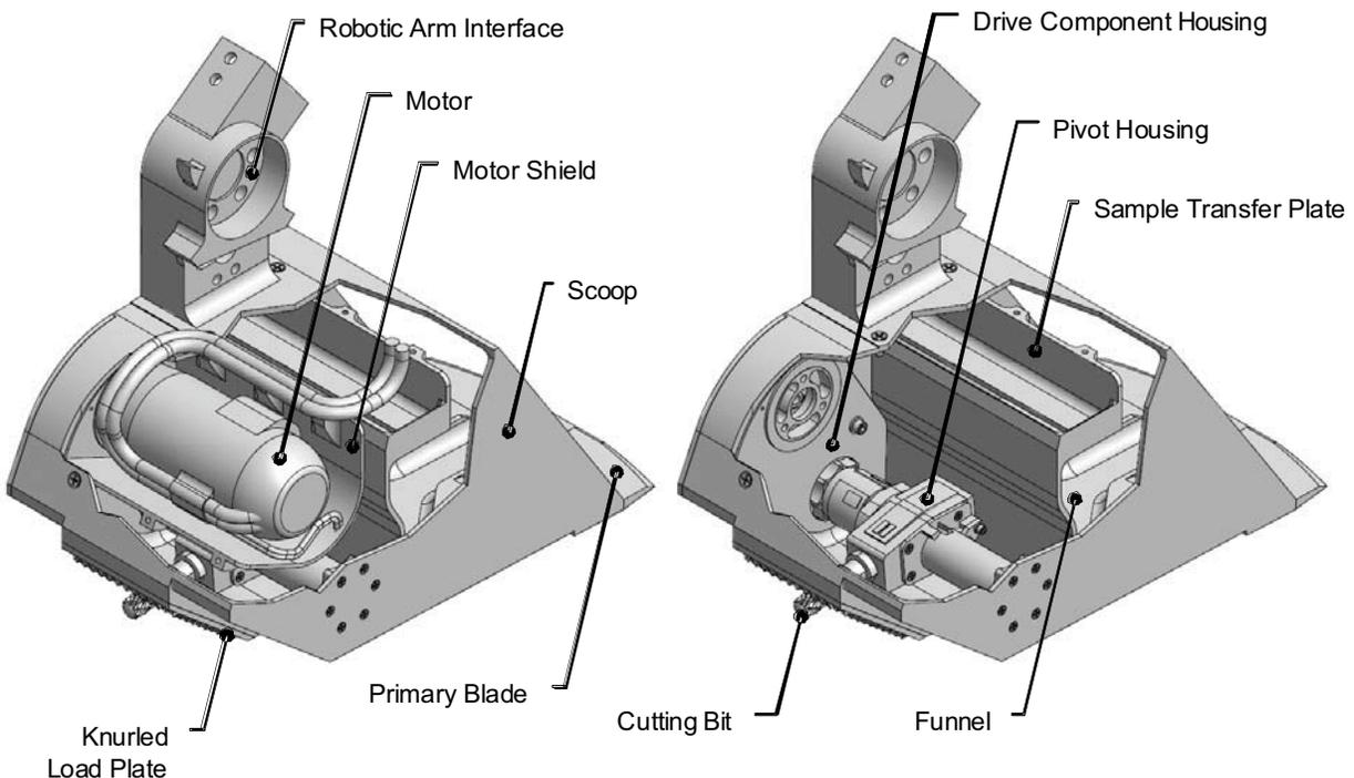
**Figure 1. Cutaway of ISAD Showing Internal Components**
