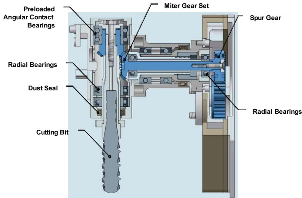
Figure 3. Drivetrain Cross Section Showing Dust Seal Location
