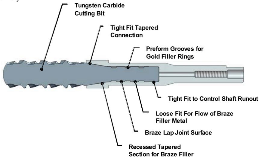
**Figure 9. Flight ISAD Cutting Bit Design**
