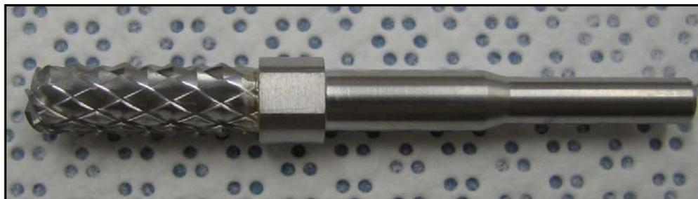
**Figure 10. Flight ISAD Braze Joint**
