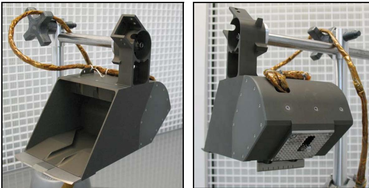
**Figure 2. Icy Soil Acquisition Device Flight Unit on Assembly Fixture**
