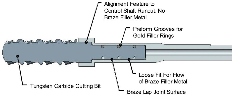
**Figure 7. Prototype Cutting Bit Braze Joint Design**
