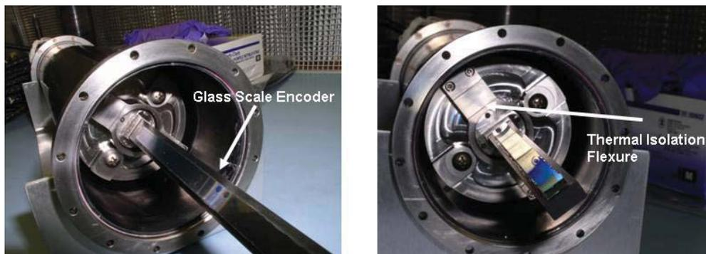
**Figure 15: Glass Scale Encoder Mount via Flexures**
