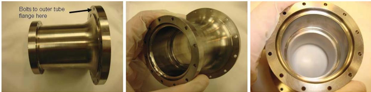
**Figure 4: Bearing Housing**
