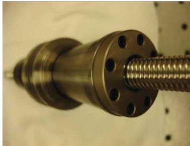
**Figure 9: Ballnut bolted to Drive Link**
