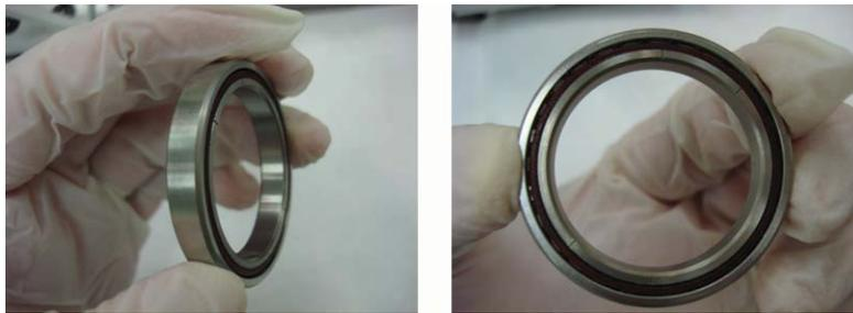
**Figure 5: Timken MPB Angular Contact Ball Bearing**
