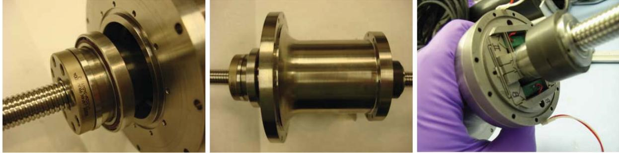
**Figure 10: Housing Assembly**
