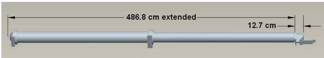
Figure 10 - Strut Rendering (Extended)
