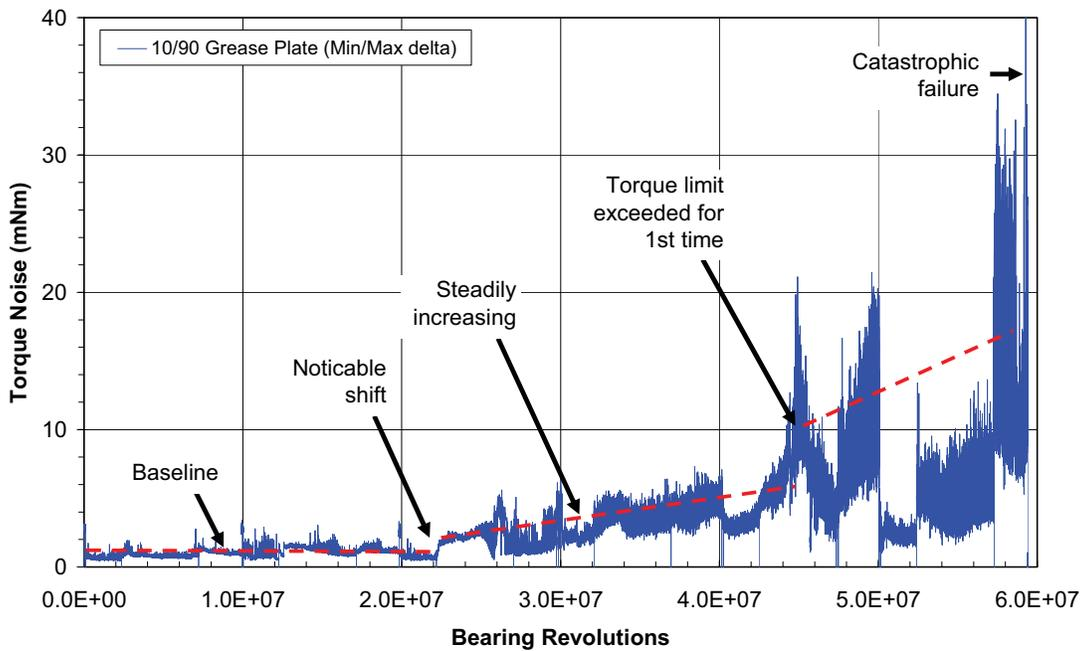
**Figure 7: Torque Noise in Grease-Plated Bearing (BP-A)**
