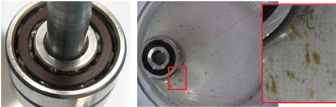
**Figure 10: BP-B Bearings Post-Test (Left – Grease-fill; Right – Flouroclean X100 soak)**
