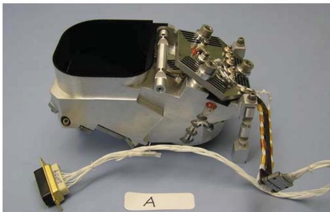
The solar calibration target is the bright plane that can be seen in Figure 3. It reflects indirect sunlight into the instrument. The black body calibration target is recessed in the yoke structure. The instrument can calibrate itself against the black body calibration target when the instrument is pointing straight down.
