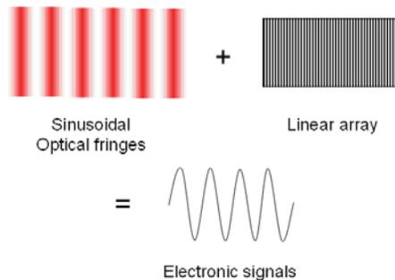
Unlike conventional encoders, small sensor-to-grating gap changes do not have a detrimental or unpredictable impact on the fringe quality. Therefore, the detector and electronics can be designed with foreknowledge of the fringe characteristics, and tuned for the very best response and filtering. In particular, the main detector array cells have been designed to filter out the third harmonic in the interference fringe pattern. These active cells are arranged in a zigzag pattern (Figure 4).
