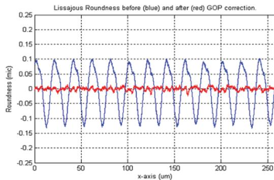
**Figure 6. Typical MII Lissajous roundness cyclic error correction**
