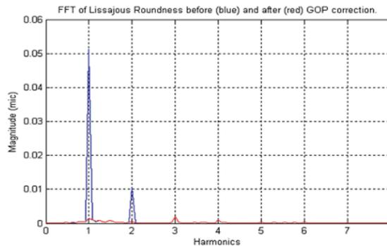
**Figure 7. Typical MII Lissajous FFT cyclic error correction**
