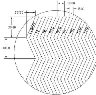
**Figure 4. Main track array (dimensions in microns)**
