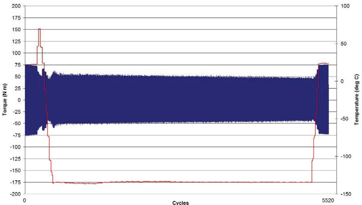
**Figure 5: Friction Torque Plot**
