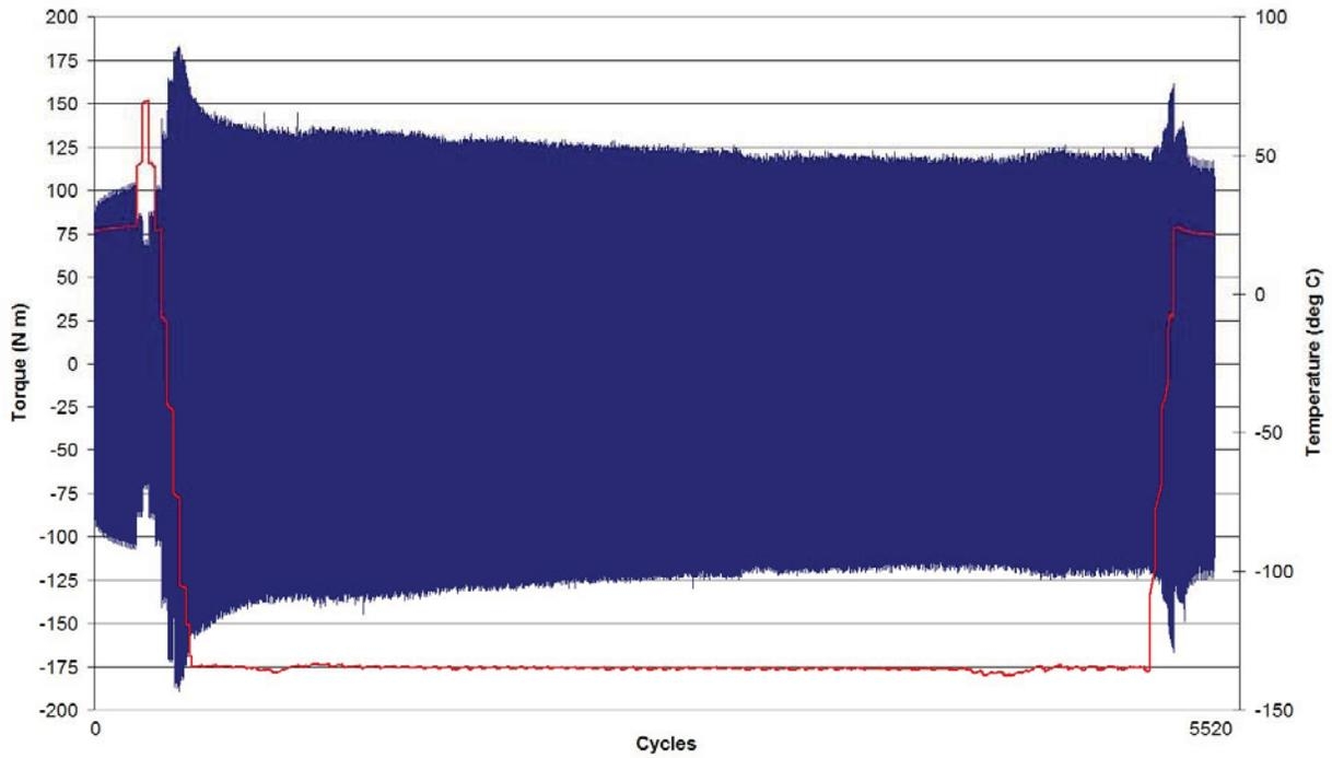
**Figure 8: Friction Torque Plot
