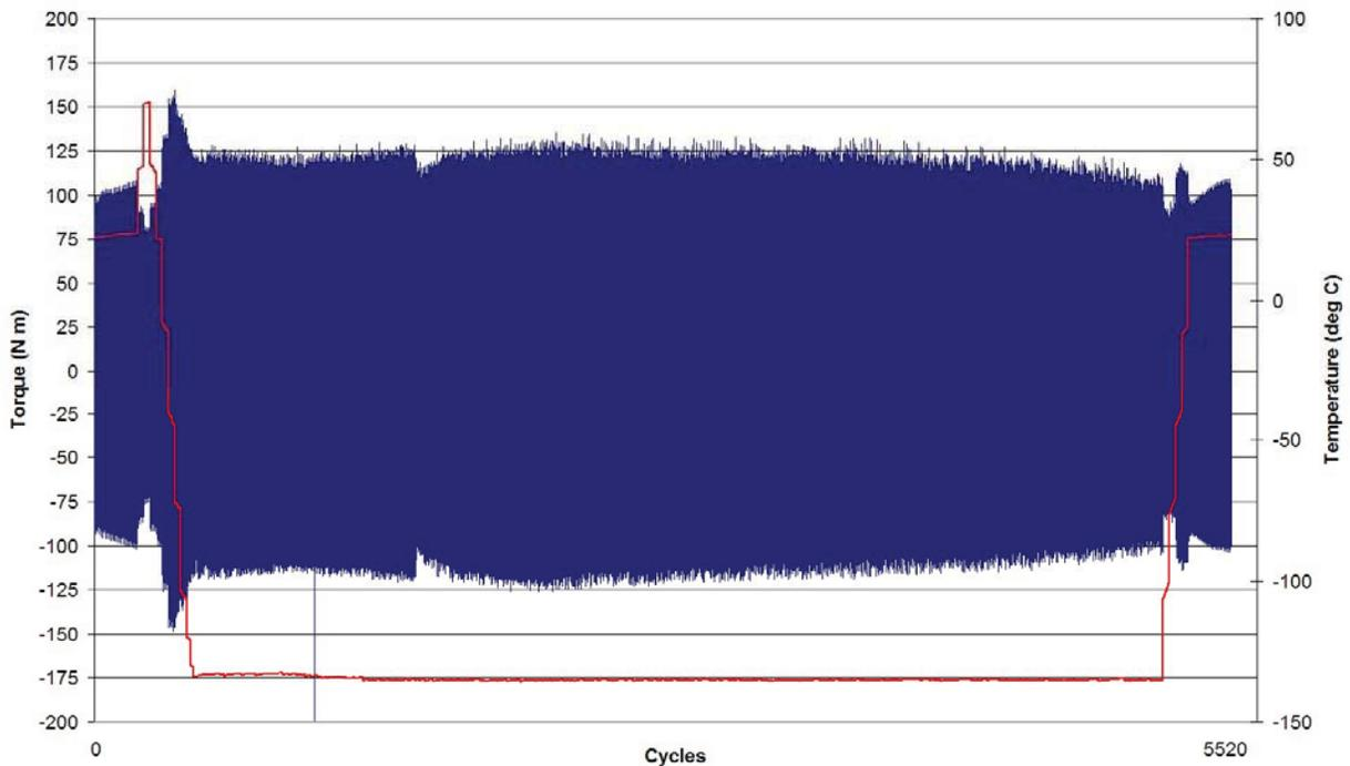
**Figure 7: Friction Torque Plot
