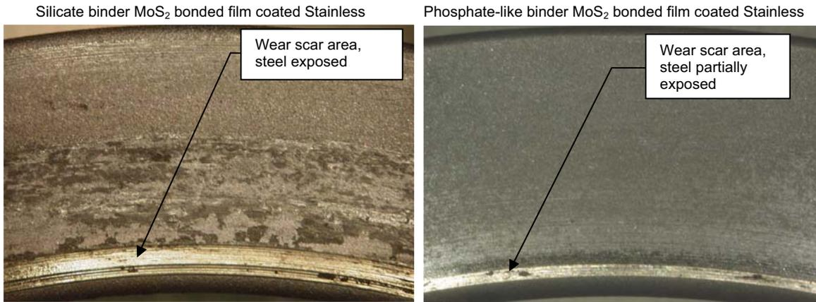
**Figure 13: Post-Test Photos of Smaller, Outboard Bushing**
