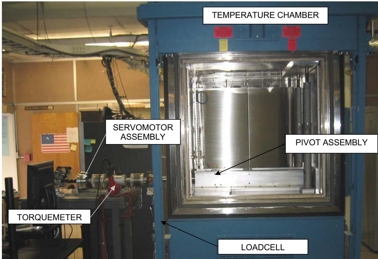
**Figure 3: Bushing Test Hardware in Temperature Chamber**
