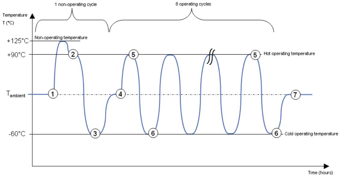
**Figure 14. Thermal cycles performed on the APS.**
