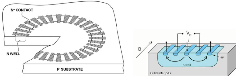
Figure 2. Integrated Hall structure and detail of a 5 Contacts Vertical Hall (5CVH) element
