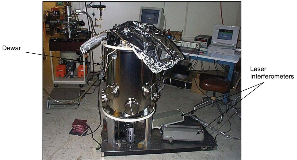
**Dewar with Laser Interferometers**
