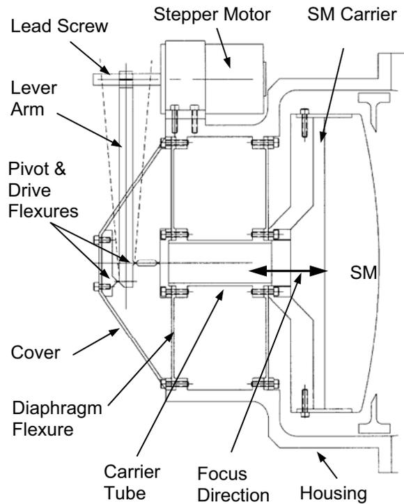
Figure 4. Focus Mechanism Concept
