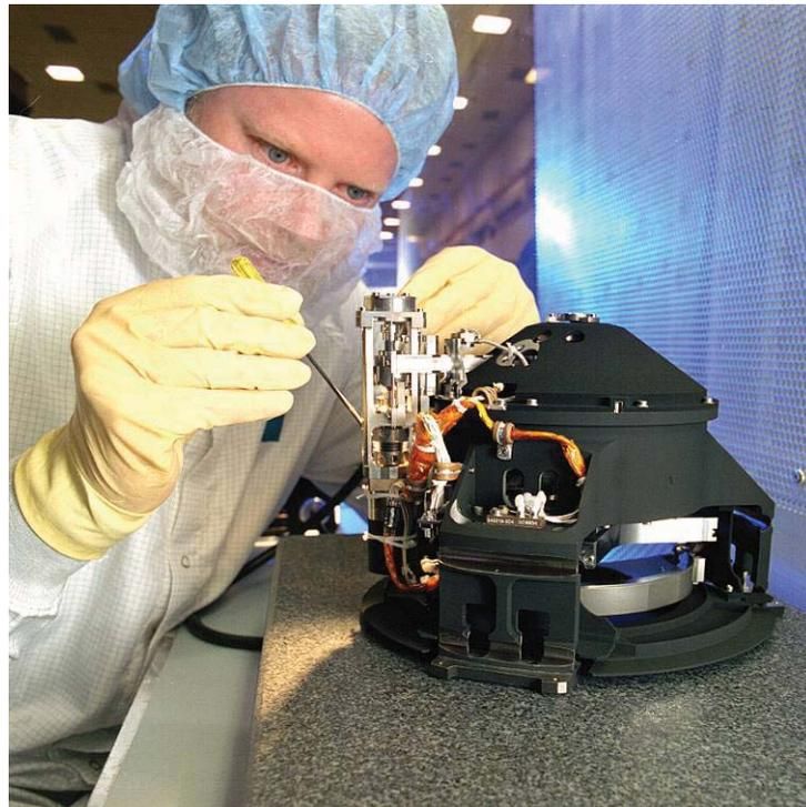
Figure 1. Flight Focus Mechanism (FLT-FM)
