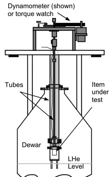
Figure 10. Component Test Set-Up
