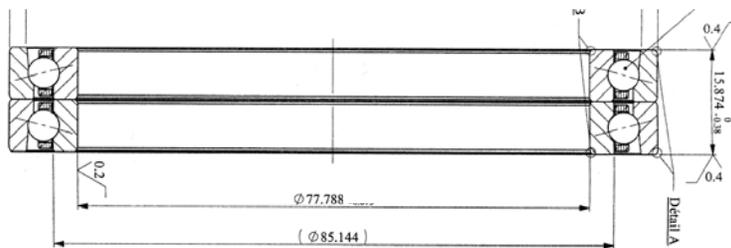
**Figure 8: Bearing Dimensions**
