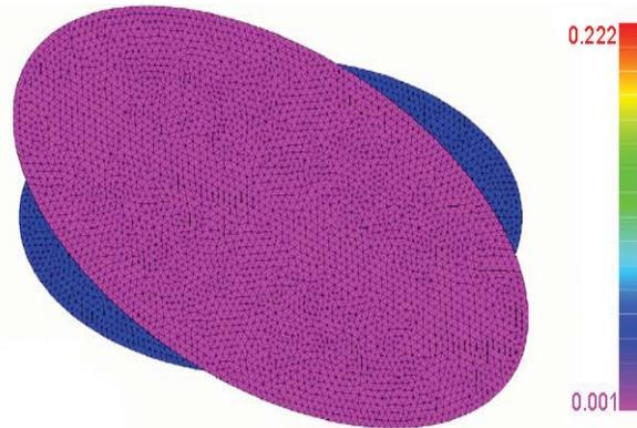
Figure 4. Mirror Mode 1, Torsional about Z-Axis, 270 Hz
