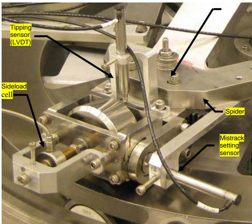
**Figure 6: Test roller with its respective instrumentation**
