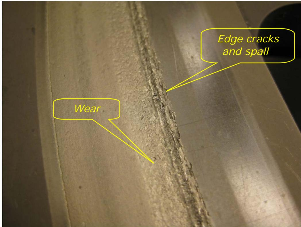
**Figure 7: Example of damage generated on outer track**
